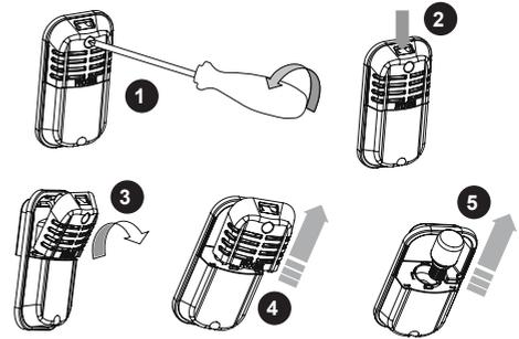
1. Remove the screw on the light cover by screw driver. (Fig.1)
